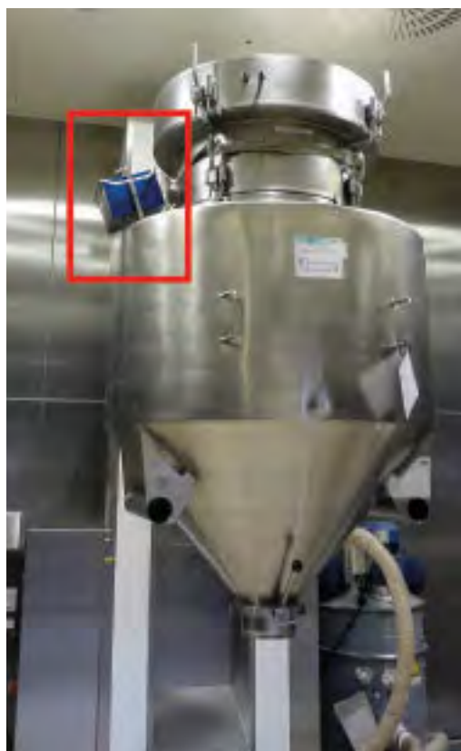
Figure 1: Production blender with the NIR instrument 'SentroPAT BU' attached
